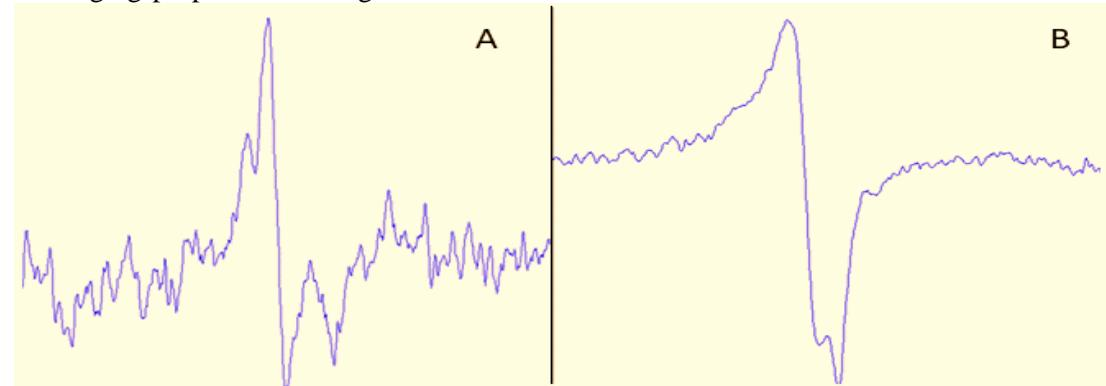
**Figure 1.** Direct EPR spectra recorded of non-irradiated (A) and UV-B/ $\gamma$ -irradiated (2.5Gy) rose oil (B).
