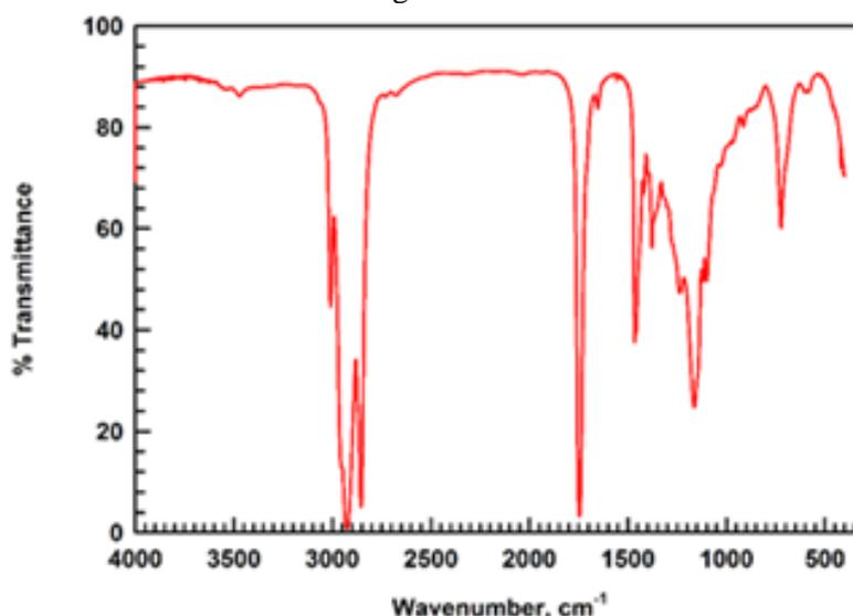
**Figure 1.** FTIR transmittance spectrum of investigated oil sample.
