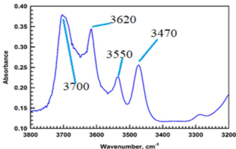
**Figure 2.** FTIR spectrum of 1%  $\text{CCl}_4$  solution of the oil in the range 3200-3800  $\text{cm}^{-1}$ .
