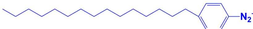
Scheme 1. Chemical structure of the probe 16\text{-ArN}_2^+ used to determine the distribution of antioxidants in oil-in-water emulsions and nanoemulsions. The counterion ( \text{BF}_4^- ) is not displayed for simplicity.
