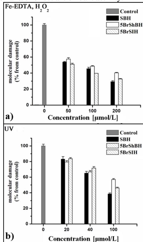
**Figure 3.** Concentration dependence of the protection effect of SBH and the studied bromo derivatives in deoxyribose containing model systems upon different mechanisms of induction of molecular damage (Fe (II) – a and UV irradiation b).
