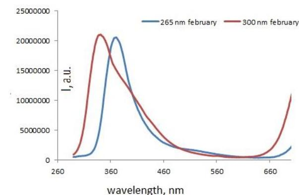
Fig. 2. Fluorescence spectra of Pinot Noir red wine excited at 265nm and 300 nm.
