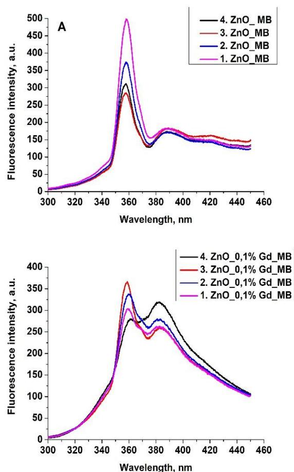
**Figure 2.** Fluorescence spectra of ZnO (A) and ZnO- $Gd^{3+}$  (B) films (0.1 mass. % Gd) under the action of myoglobin. Myoglobin concentration in solution for depositing on films surfaces: **1** –  $10^{-6}$ , **2** –  $10^{-8}$ , **3** –  $10^{-10}$ , **4** –  $10^{-12}$  M.
