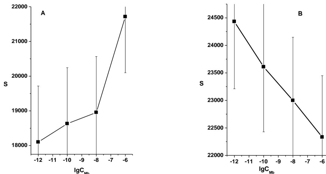
**Figure 3.** Dependence of the fluorescence intensity on the myoglobin concentration for ZnO (A) and ZnO-Gd<sup>3+</sup> films (B).
