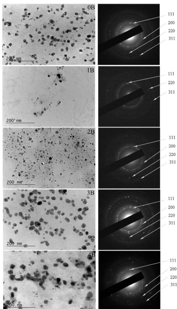
**Figure 3.** TEM analysis of AgNPs. The sample numbers are according to Table 1.
