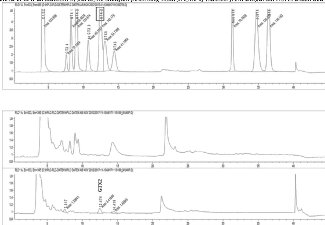
**Fig. 3.** HPLC-FD with post column derivatization PCOX chromatograms of a PSP standard mix containing B1, C1/2, GTX1-4, dcGTX2/3, NEO, dcSTX and STX(top) and extract of cultured mussel sample MU48P without derivatization (middle) and with derivatization (bottom).
