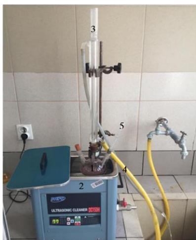
**Figure 1.** Experimental setup for ultrasound leaching.
