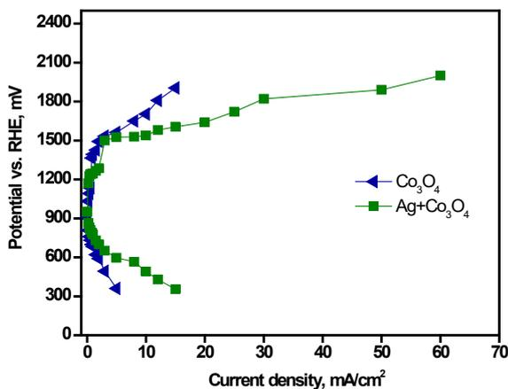
**Figure 6.** Polarization curves of the electrodes for ORR and OER for catalysts: ■ Ag +  $\text{Co}_3\text{O}_4$ ; ▼  $\text{Co}_3\text{O}_4$ . The electrolyte was 6 M KOH at room temperature. The geometrical area of the electrode was  $25 \text{ cm}^2$ .
