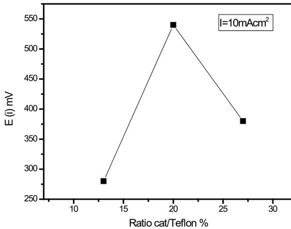
**Figure 5.** Optimization curve of the ratio for ORR (catalyst – PTFE at a constant catalytic mass amount =  $40 \text{ mg/cm}^2$ ).
