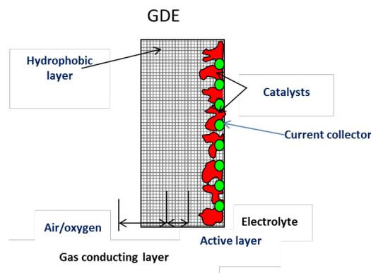
**Figure 1.** Schematic cross-section of the air gas diffusion electrode.
