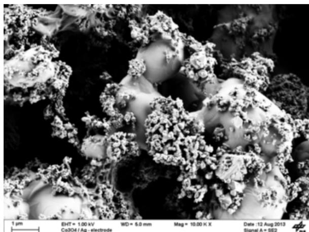
**Figure 2.** SEM picture of an Ag /Co<sub>3</sub>O<sub>4</sub> mixture.
