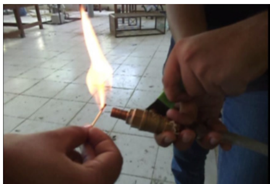
Fig. 8. Flame test of cow dung and sewage water
