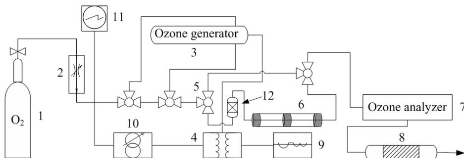
**Fig. 1.** Experimental set-up for catalytic decomposition of ozone: 1 - oxygen; 2 - flow controller; 3 - ozone generator; 4 - transformer; 5 - three-way stopcock; 6 - reactor charged with catalyst sample; 7 - ozone analyzer; 8 - reactor for decomposition of residual ozone; 9 - current stabilizer; 10 - autotransformer; 11 - voltmeter; 12 - moisturizer.
