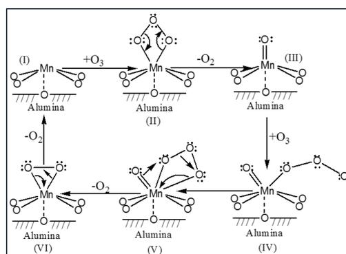
Fig. 4. Mechanism of ozone decomposition on MnO<sub>x</sub>/Al<sub>2</sub>O<sub>3</sub> catalyst.
