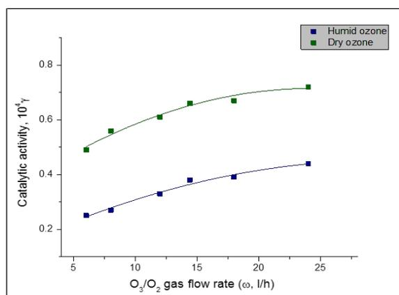
Fig. 3. Flow rate dependence on catalytic activity in dry and humid reaction environment.
