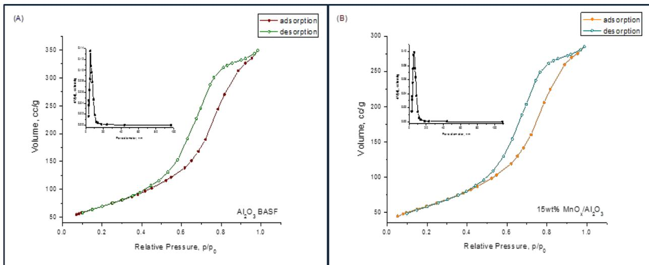
Fig. 5. Nitrogen adsorption-desorption isotherms of pure  $\text{Al}_2\text{O}_3$  (a) and 15 wt%  $\text{MnO}_x/\text{Al}_2\text{O}_3$  catalyst (b)
