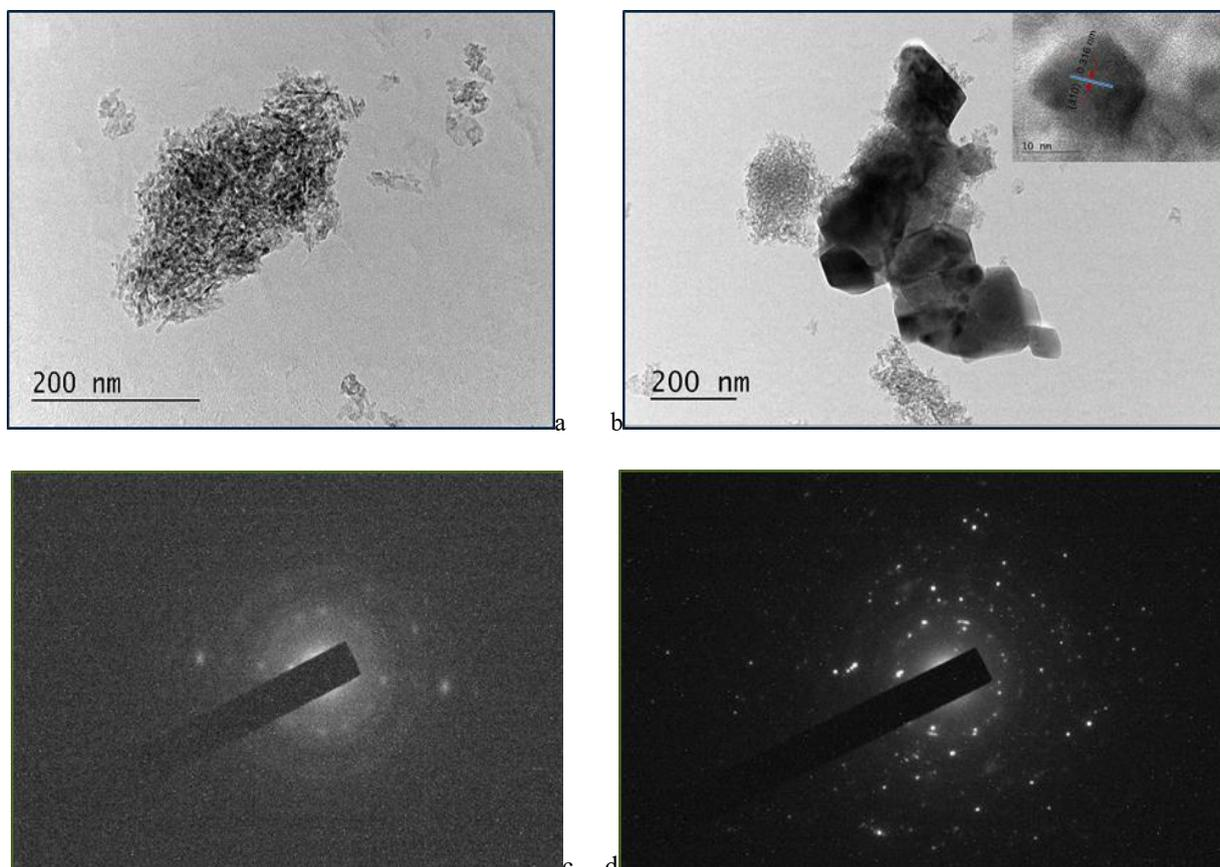
Fig. 6. HRTEM images of  $\text{Al}_2\text{O}_3$  (a) and  $\text{MnO}_x/\text{Al}_2\text{O}_3$  catalyst (b); SAED patterns of  $\text{Al}_2\text{O}_3$  (c) and  $\text{MnO}_x/\text{Al}_2\text{O}_3$  catalyst (d).
