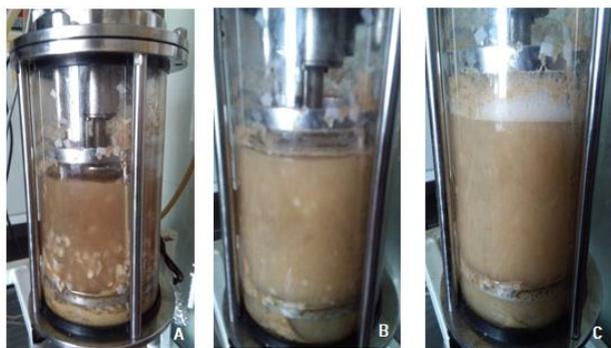
**Fig. 1.** Microbial degradation of filter paper pieces: at the beginning of the process (A), after 15 days (B) and after 20 days (C).
