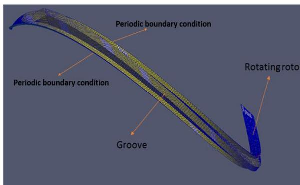
**Fig. 14.** Geometry and mesh of helix groove
