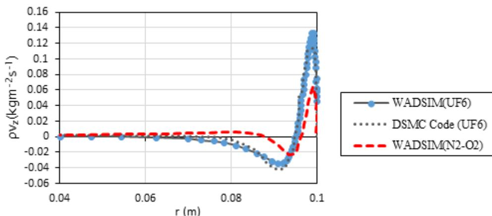
Fig. 13. Axial mass fluxes of air and UF<sub>6</sub> using the WADSIM\_1 software and DSMC code
