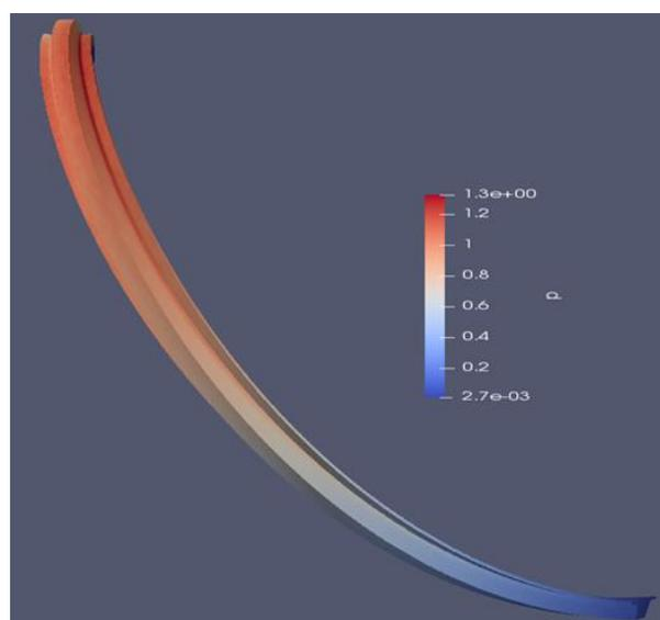
**Fig. 15.** The contour of pressure variations (Pa) along the groove length using WADSIM\_1 software
