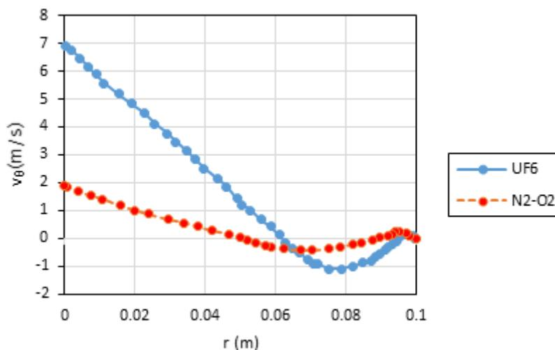
Fig. 12. Axial velocities of air and UF<sub>6</sub>
