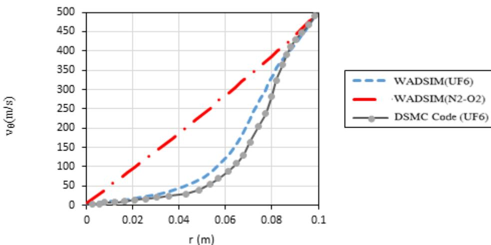
Fig. 11. Azimuthal velocity of air and UF<sub>6</sub> using WADSIM\_1 software and DSMC code
