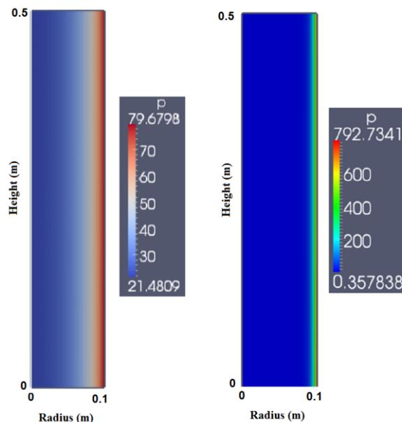
Fig. 8. Contours pressure for air and UF<sub>6</sub>
