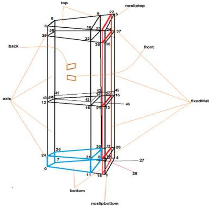
Fig. 4. The simulated geometry and its elements and boundaries
