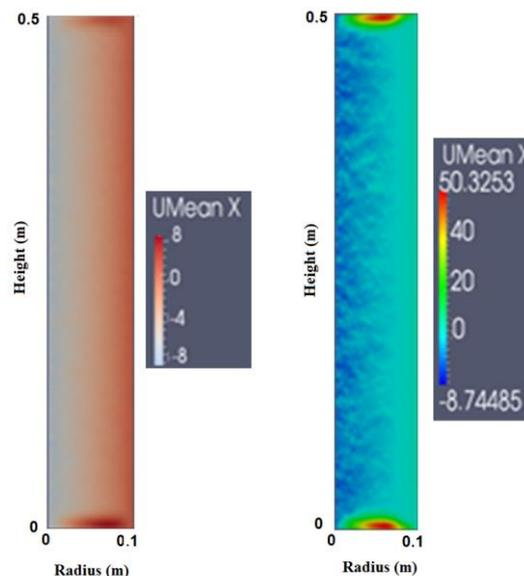
Fig. 10. Radial velocity contour for air and UF<sub>6</sub>
