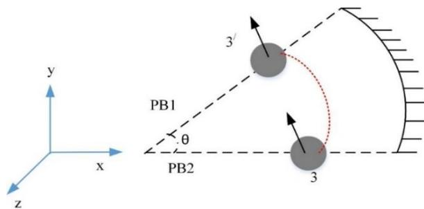
Fig. 3. A schematic of a periodic boundary condition in a rotational transform
