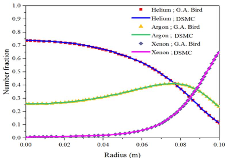
Fig. 7. Comparison of the number density profiles obtained from the two-dimensional DSMC code and the one-dimensional code of Bird [3].
