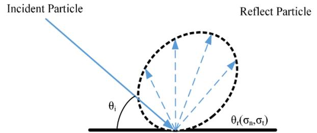
Fig. 2. Incident and reflected particle scheme in the Cercignani-Lampis-Lord model
