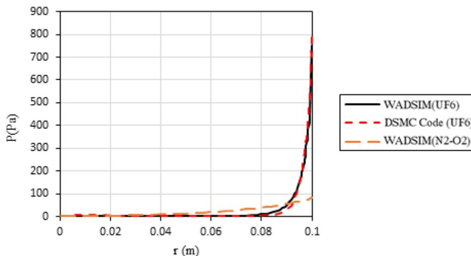
Fig. 9. The radial pressure distribution for air and UF<sub>6</sub> using WADSIM\_1 software and DSMC code.
