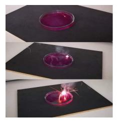
It is observed that the batch of sodium is bounced on the water and that the water is colored in a raspberry color. When potassium reacts with water the reaction is more violent, a flame is being observed on the surface of the water.
