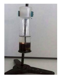
Small flashes are observed at the boundary between the two layers. There is a clear crack.
