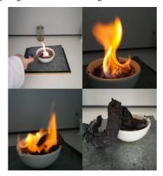
Carbonization of sugar and simultaneous decomposition of the baking soda is observed by the release of carbon dioxide, which gives volume to the resulting mass. As a result, the volume of the mixture is increased several times and crawling of a "snake" in black color is observed.
