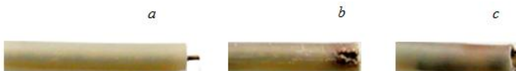
Fig. 1. Cable-electrode and characteristic failures during its operation (a) before treatment, (b) at W = 600 J, and (c) at W = 1350 J.
