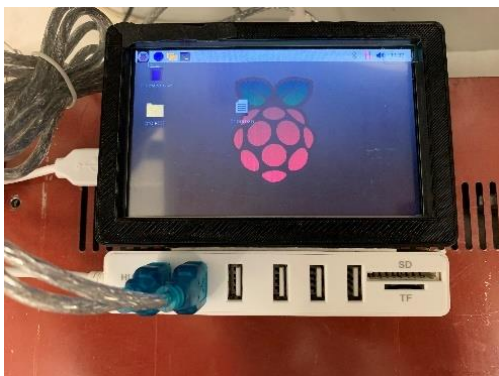
Fig.5. The Raspberry-Pi is connected to instruments via USB ports and stored in a 3-D printed box (designed using Open-Scad)
