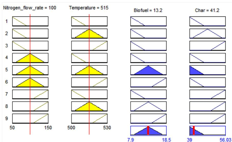
**Figure 5.** Ruler view of input variables (nitrogen flow rate and temperature) with output variables (biofuel and char)
