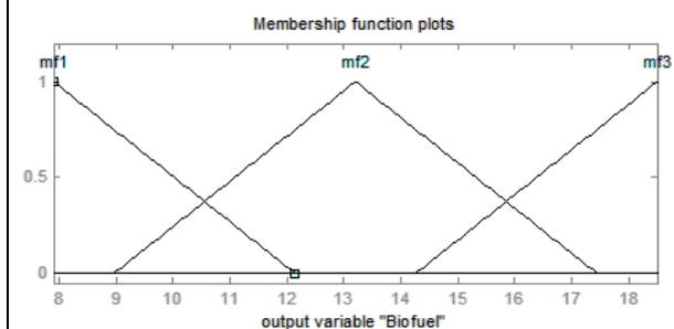
**Figure 4 (a).** Fuzzy model of thermochemical (mamdani) showing output variable biofuel.
