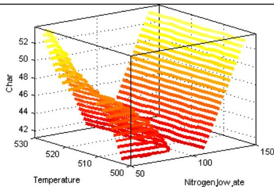
**Figure 6 (b).** Control surface view of the fuzzy model with nitrogen flow rate, temperature vs. char
