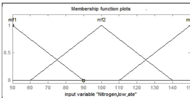
**Figure 3 (a).** Fuzzy model of thermochemical (mamdani) showing input variable nitrogen flow rate.
