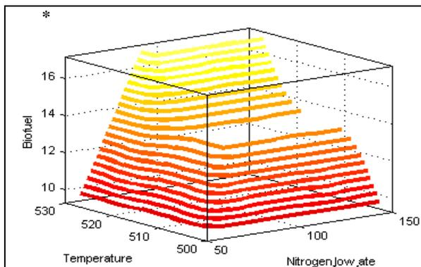
**Figure 6 (a).** Control surface view of the fuzzy model with nitrogen flow rate, temperature vs. biofuel
