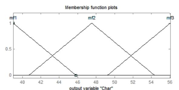
**Figure 4(b).** Fuzzy model of thermochemical (mamdani) showing output variable char.
