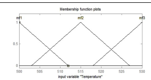
**Figure 3 (b).** Fuzzy model of thermochemical (mamdani) showing input variable temperature.
