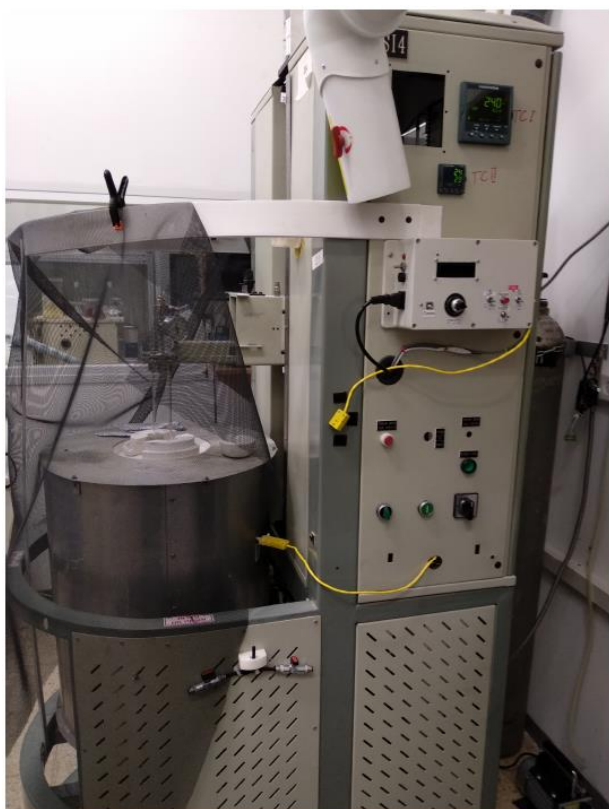
Fig.1. Bridgman based growth furnace with a quartz compartment for growing the crystals in an inert environment
