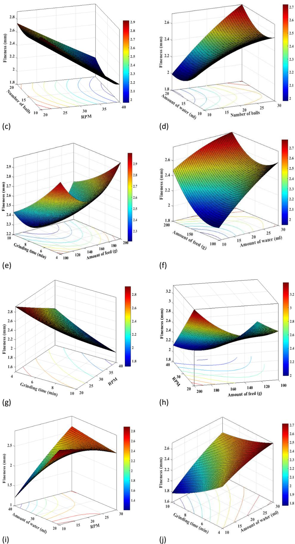
Figure 2 (a - j) 3D plots of wet grinding independent parameters with their response as fineness of coal.
