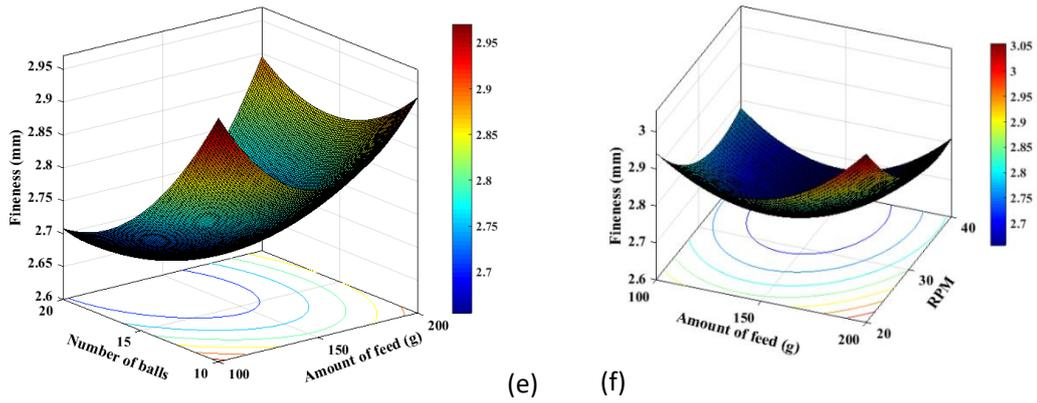
**Figure 1** (a-f) 3D plots of all four parameters combination effect on response as fineness of coal.
