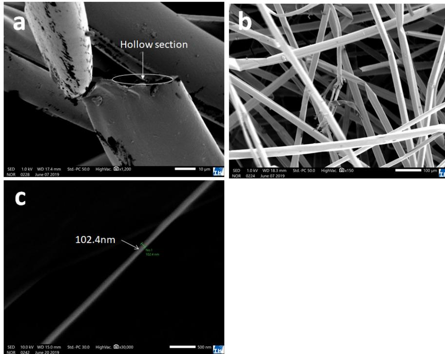
Figure 2. SEM micrographs of *Calotropis Procera* seed fiber at magnification (a)×1200, (b) ×150 and (c) ×30000
