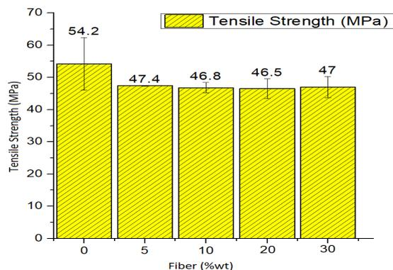
**Figure 6.** Tensile strength of composites for pure PLA, 5%, 10%, 20% and 30% fiber content
