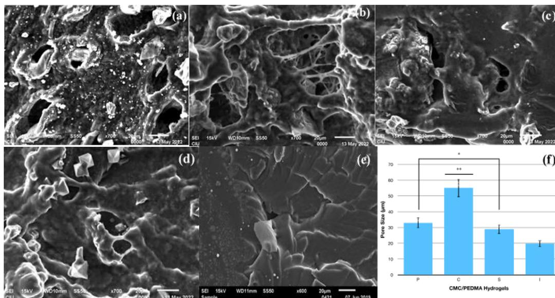
**Figure 4.** SEM results of (a) P, (b) C, (c) S, (d) I, (e) PEGDMA without CMC and (f) pore size distribution of /CMCPEGDMA hydrogels.
