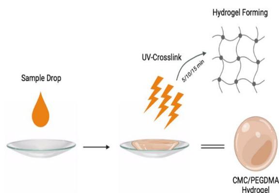
**Figure 1.** Schematic photopolymerization process of the hydrogels
