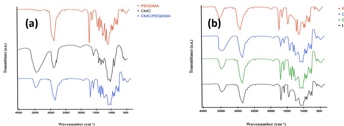
**Figure 3.** FTIR results of (a) PEGDMA, CMC and CMC/PEGDMA blend, (b) P, C, S and I.
