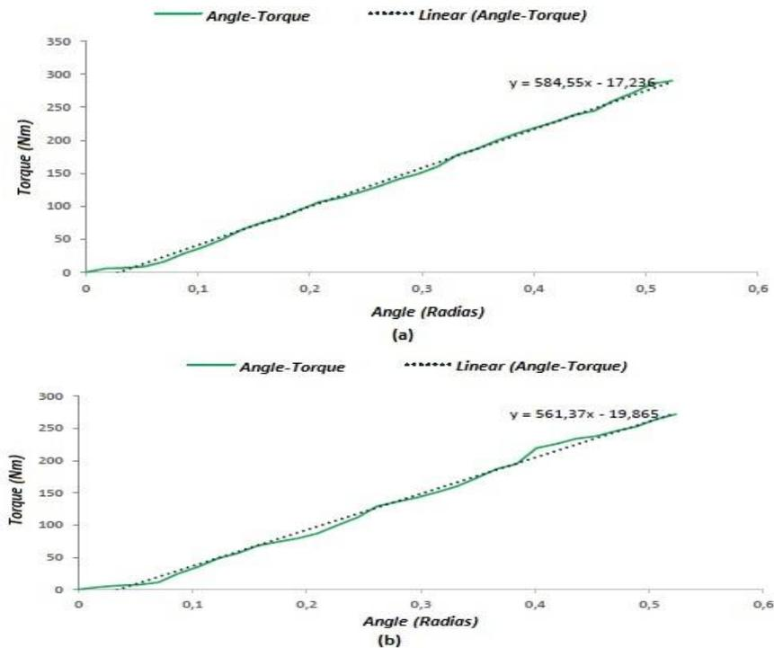
Fig. 5. Angle-torque graph of a) nanoalumina-reinforced b) nanozeolite-reinforced NR rubber crank pulley by spraying method
