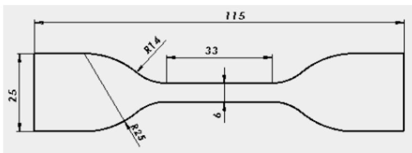
**Fig. 2.** ASTM D412 – C sample type
