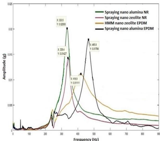
Fig. 7. Natural frequency test results of sample pulleys
