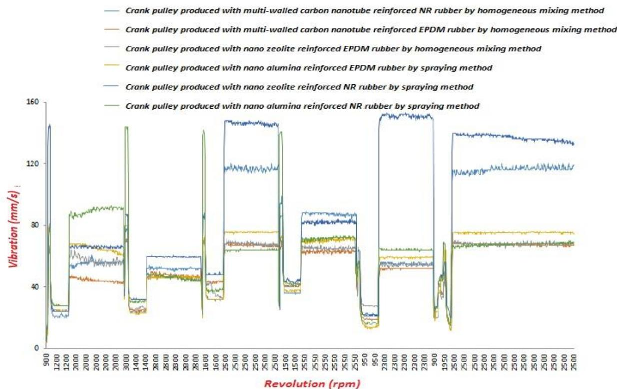
Fig. 8. Speed – vibration test results of sample pulleys
