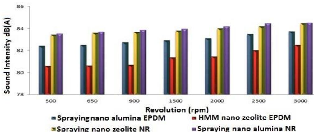
Fig. 9. Sound intensities of sample pulleys
