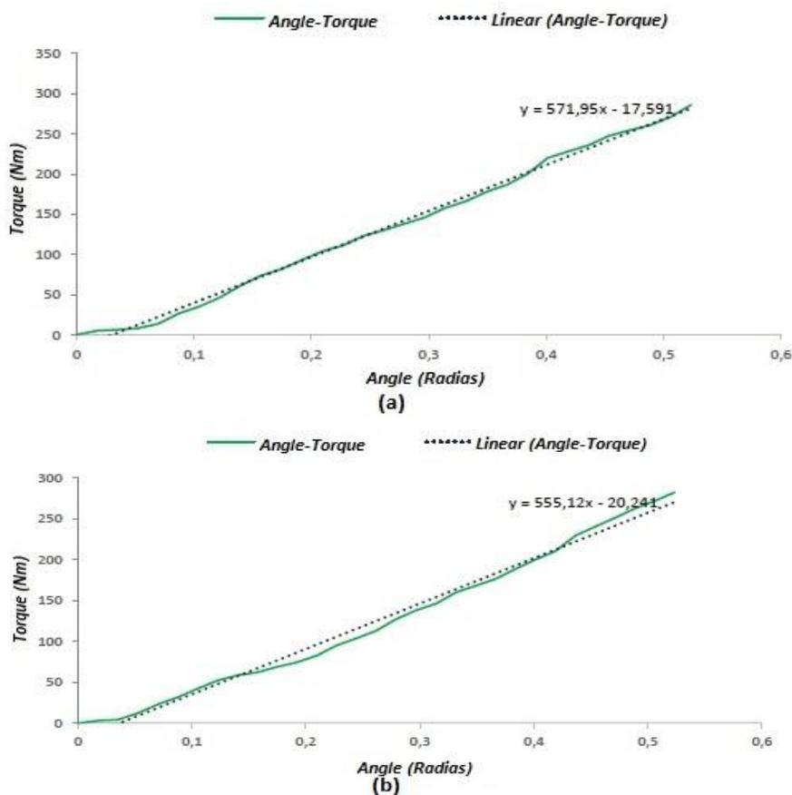
**Fig. 6.** HMM of EPDM rubber a) reinforced with nanozeolite and b) reinforced with nanoalumina by spraying method. Angle-torque graph of the crank pulley
