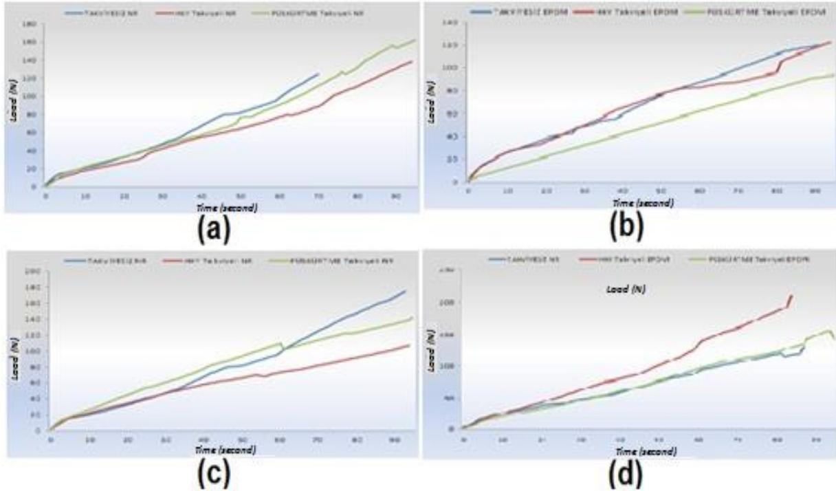
Fig. 4. Uniaxial tensile test results of sample rubbers
