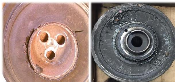
Fig. 1. Defects in the crank pulley
