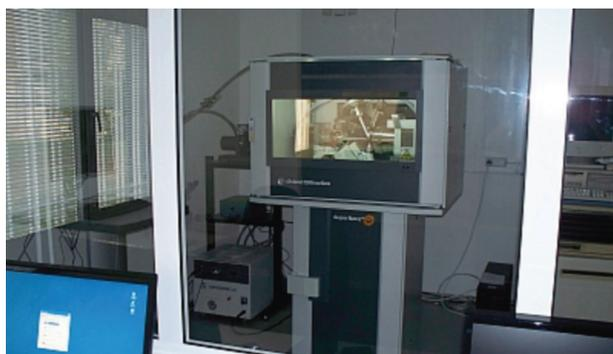
**Fig. 3.** The X-ray single crystal diffractometer Supernova A (Oxford Diffraction) in the Laboratory of X-ray diffraction analysis, IMC (2010).
