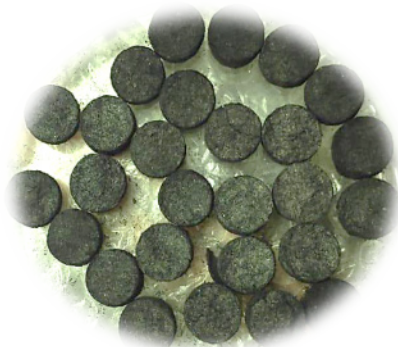
Figure 1. Granulated activated carbon obtained from rice husk, oil sludge and gelatin at a ratio of 9: 1: 2.
