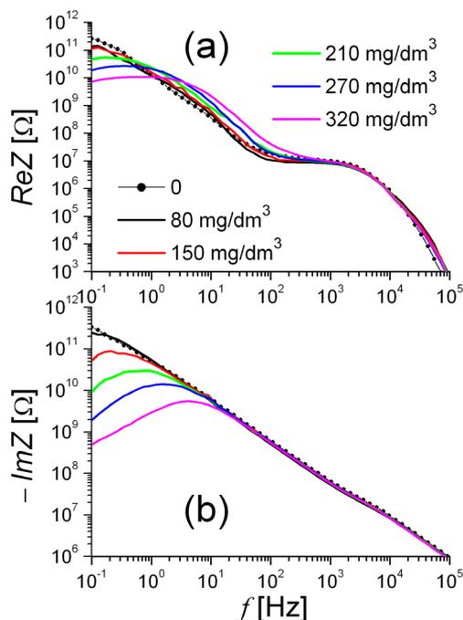
**Fig. 2.** Frequency spectra of real  $ReZ$  (a) and imaginary  $ImZ$  (b) parts of complex electrical impedances measured for DPPE LB film deposited on interdigital electrodes, being exposed to methanol vapors. The concentrations ( $\text{mg}/\text{dm}^3$ ) of the vapors are given; 0 corresponds to methanol gas-free case. The temperature was  $26^\circ\text{C}$ .
