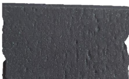
**Fig. 3.** Sintered Ni electrode
