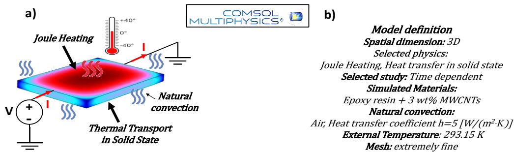
Figure 3. a) Case study addressed in the present study; b) Main model definitions for the numerical investigation adopted in COMSOL Multiphysics
