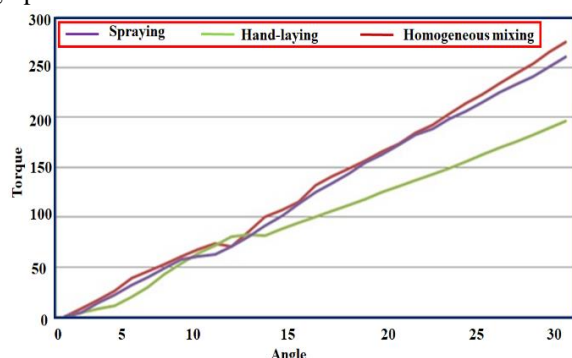
Fig. 6. EPDM rubber angle-torque graph with MWCTs reinforcement
