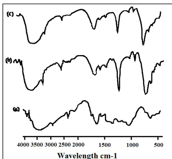
Fig. 1. FTIR spectra (a) St-g-PMA (b) St-g-PMA-g-PVA (c) PVA
