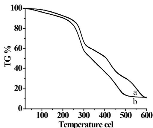
Fig. 1. Comparative TGA graph of St-g-PMA (b) St-g-PMA-g-PVA (a).
