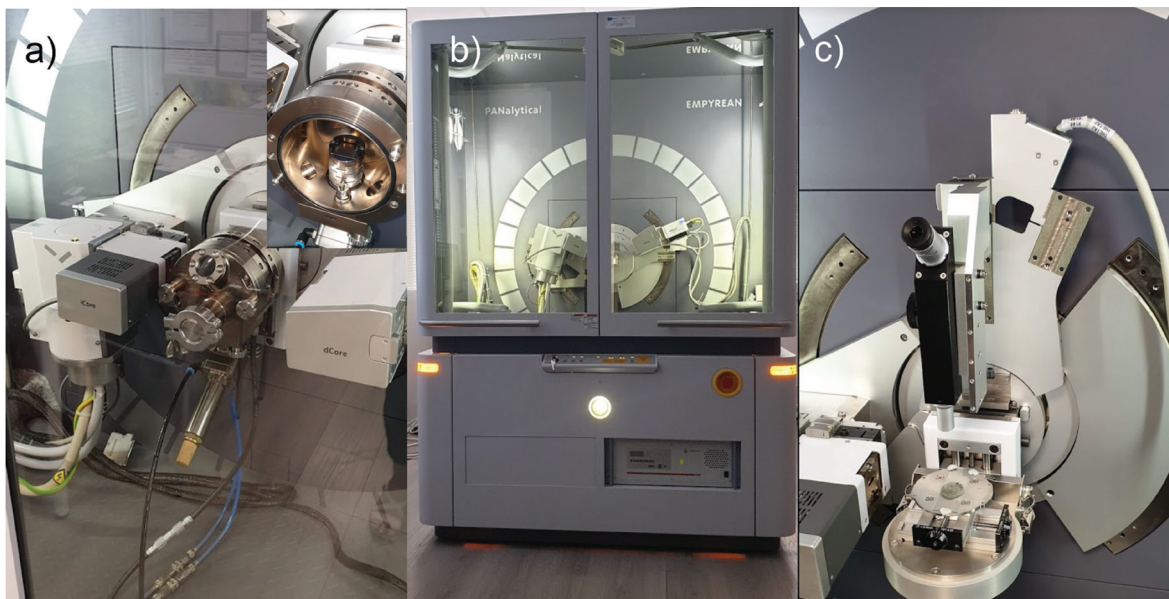
Figure 10. Diffractometer Empyrean. Applications: qualitative phase/polymorphs and quantitative analysis (wt%), Cu (1.5406 Å) and Co (1.7902 Å) sources; modes: reflection, transmission, microdiffraction (spot of 50 μm), measurements at different temperatures and different gas environments, low temperature (to -200 °C), high-temperature (to +600 °C), controlled atmosphere, SAXS/USAX, thin layers (up to 500 nm), microdiffraction, xyz stage etc.
