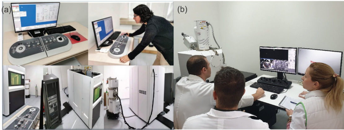
Figure 1. Installed (a) FEI 200 cryo-transmission electron microscope (cryoTEM) and (b) scanning electron microscope at the laboratory of Drug delivery systems for targeted effect of drugs and personalized medicine – MU Plovdiv.
