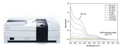
**Figure 14.** UV-VIS Cary 4000, range 175–900 nm; works with solid and liquid sample solid volume  $\sim 1 \text{ cm}^3$ , liquid sample volume from 0.2 to 3.5 ml; the system is optimal for analyzing solid samples or liquid biological samples with minimal sample preparation. Monitoring drug release, degradation, sedimentation, comparing solutions *vs* solid state in APIs.
