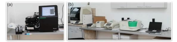
Figure 2. Major infrastructure and equipment at the laboratory "Molecular genetic markers for medical use" (a) next generation sequencer and (b) digital droplet PCR system.
