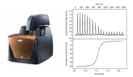
**Figure 12.** Affinity ITC, TA Instruments – detects interaction between protein/DNA/antibody and drug (ligand), works with solutions, cell volume (190  $\mu$ l), syringe volume (250  $\mu$ l), temperature range (2–80 °C), measured heat range (0.04–5000  $\mu$ J).
