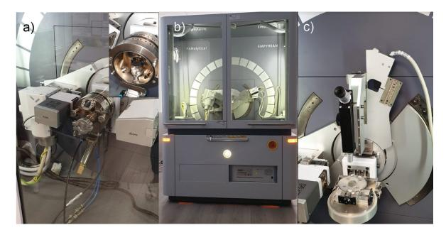
**Figure 10.** Diffractometer Empyrean. Applications: qualitative phase/polymorphs and quantitative analysis (wt%), Cu (1.5406 Å) and Co (1.7902 Å) sources; modes: reflection, transmission, microdiffraction (spot of 50  $\mu$ m), measurements at different temperatures and different gas environments, low temperature (to –200 °C), high-temperature (to +600 °C), controlled atmosphere, SAXS/USAX, thin layers (up to 500 nm), microdiffraction, xyz stage etc.
