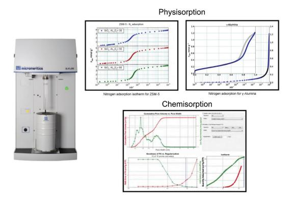
Figure 13. Surface area analyzer – BET, 3Flex Micromeritics: nanopowders surface area, detects the loading of drugs on nanocarriers, determines surface are, pores sizes.
