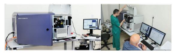
Figure 3. Cell Sorter based on 4 laser multiparameter flow cytometry.
