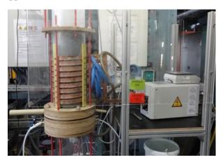
**Figure 2.** Picture of the cylindrical fluidized bed apparatus from Figure 1. Shows the fluidized bed chamber surrounded with the copper induction coil.
