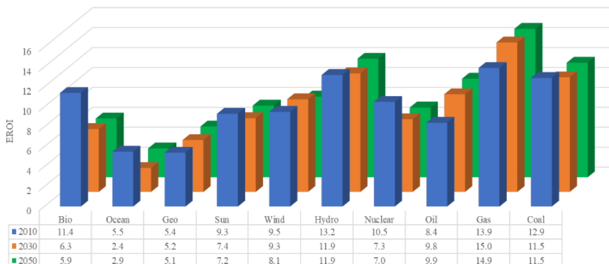
Fig. 1. Forecast of global average EROI for various types of energy resources until 2050
