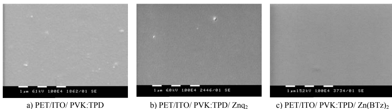
Fig. 19. SEM micrographs of PET/ITO/PVK:TPD, PET/ITO/PVK:TPD/ \text{Znq}_2 , and PET/ITO/PVK:TPD/ \text{Zn}(\text{BTz})_2 surfaces.
