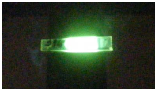
Fig. 22. Picture of our luminous OLED device with structure ITO/(PVK:TPD _{20} )/Zn(BTz) _2 /Al at 15 V DC.
