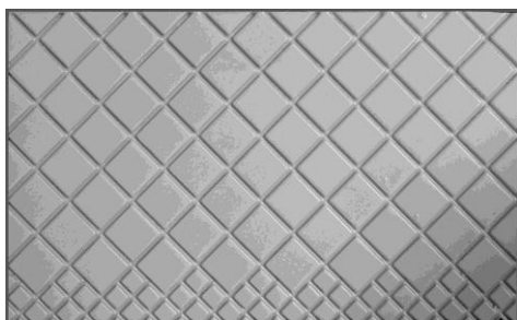
Fig. 2. Polystyrene packing plate with stamped inclined capillary grooves.
