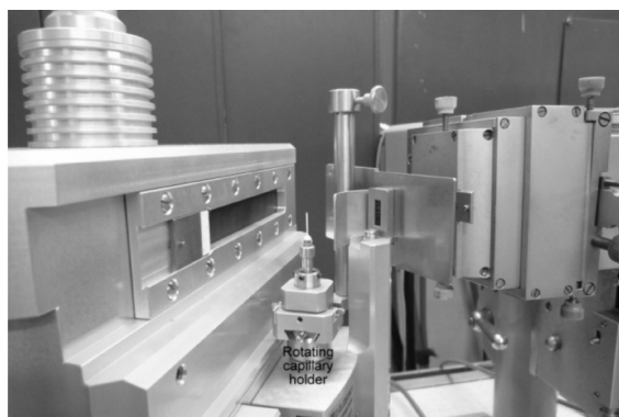
Fig. 2. Rotating capillary setup
