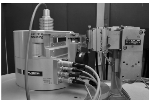
Fig. 1. Swinging flat sample setup
