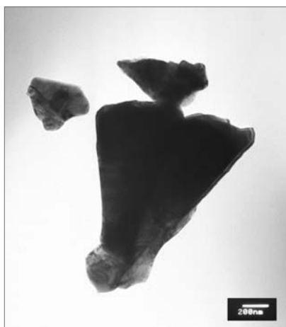
Fig. 3. TEM photograph of ZnO prepared by the decomposition method
