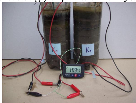
Fig. 5. Connected in series SMFCs supplying digital watch
