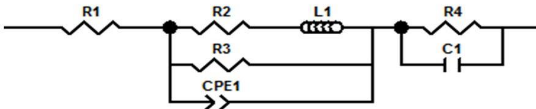
Fig. 5 Equivalent circuit according to the surface charge approach [14]. R_1 – electrolyte resistance, R_2 – surface charge resistance, L_1 – surface charge pseudo-inductance, R_3 – ion migration resistance, CPE_1 – oxide capacitance generalized in the form of a constant phase element, R_4 – charge transfer resistance at the film/solution interface, C_1 – faradaic and/or adsorption pseudo-capacitance.
