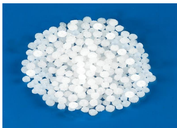
Fig.1. Modified nitrogen fertilizer granules with PVA-M membrane
