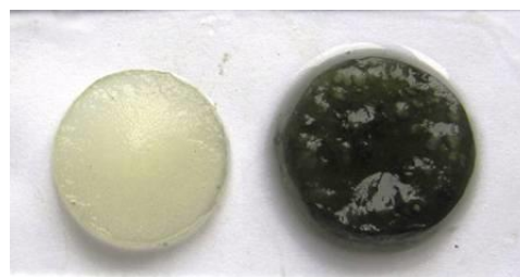
Fig. 6. Digital image of the matrix without cells (left) and the matrix with entrapped cells (right)
