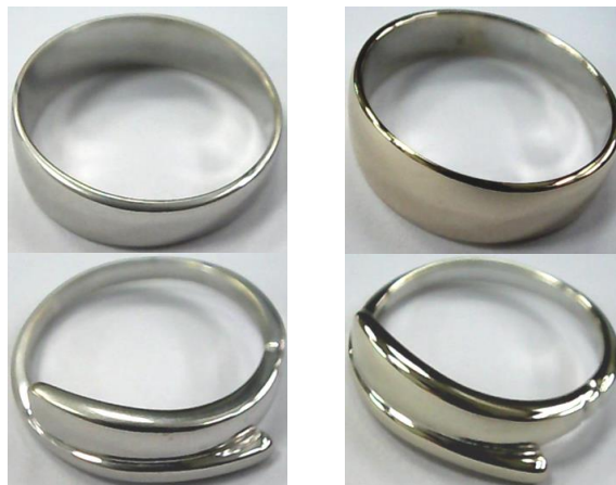
Picture 1. Products before and after coating with a layer of semi-finished rhodium
