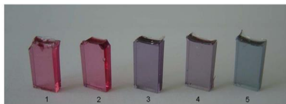
Fig. 1. Au/urea silicate samples with different degree of Au NPs aggregation.
