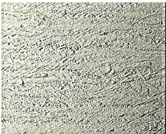
Fig. 4. Microstructure of cold rolled and aged specimen of white alloy Au585Ag65Cu277Zn16Pd57 at 300°C, 30 min, twins, longitudinal direction, \times 500 .
