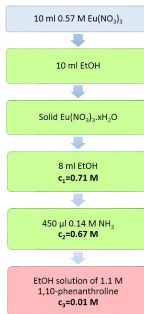
Fig. 1. Preparation of colloidal solution of [\text{Eu}(\text{phen})_2](\text{NO}_3)_3 \cdot x\text{H}_2\text{O} . The calculated Eu concentration is given in the different steps of preparation.
