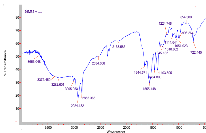
Fig. 7. FTIR spectrum of GMO, obtained from WG with catalyst TiAl and after neutralization of the remained acids with alcohol solution of methylamine.
