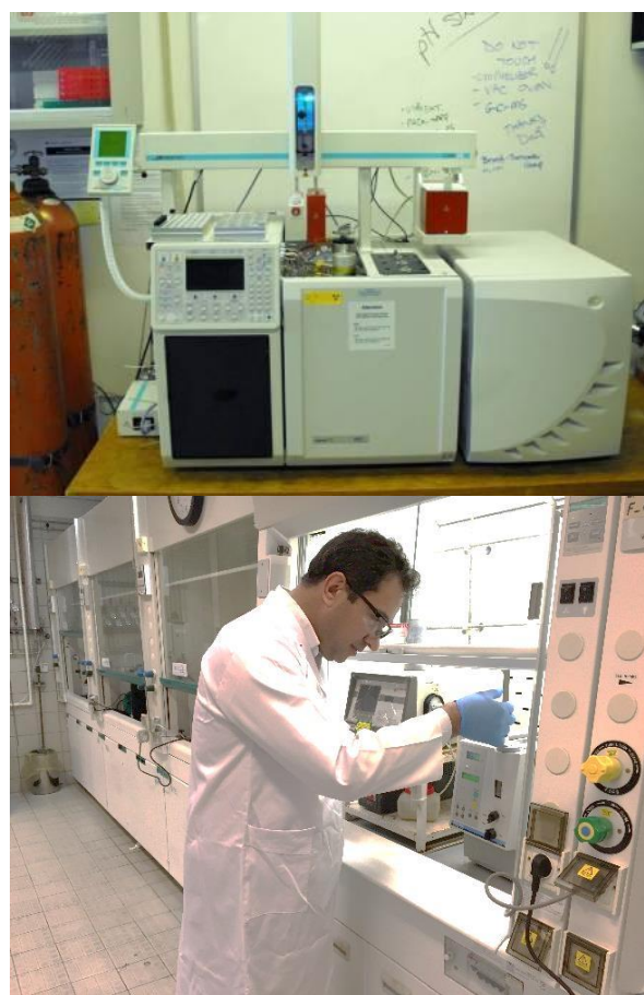
Fig. 4. GC- FID test equipment and lab experts.
