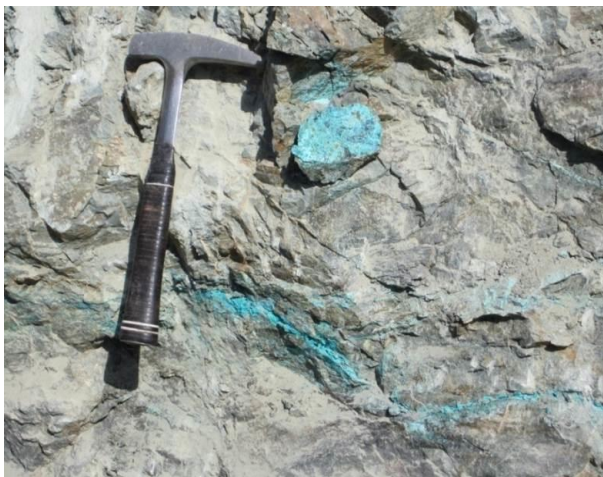
Fig. 8. Malachite mineralization in oxidation zone of Mazayjan Cu deposit, greenschist of Suriyan metamorphic complex was host rock of this mineralization.
