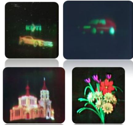
Fig. 5. Photographs of reconstruction from printed holograms.
