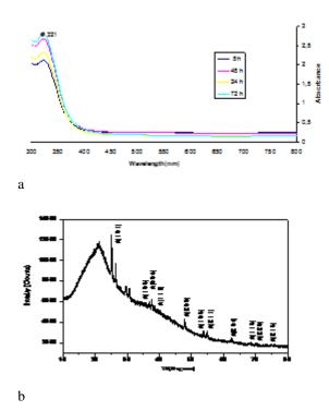
**Fig. 1.** a) UV-Vis absorption spectrum of  $TiO_2$  nanoparticles from water extract of *A.anthodium* b) XRD patterns of synthesized  $TiO_2$  nanoparticles
