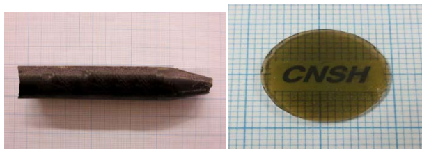
Fig. 2. CNSH cylindrical crystal (a) after removing from ampoule and (b) Cut and polished piece.
