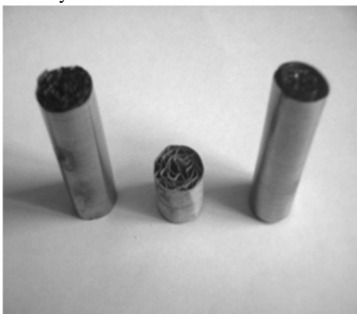
Fig. 1. Laboratory samples of neutralizers on metal blocks
